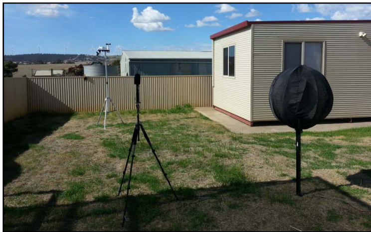
Figure 1 – Picture of the EPA microphones and weather station at the “township” site.
