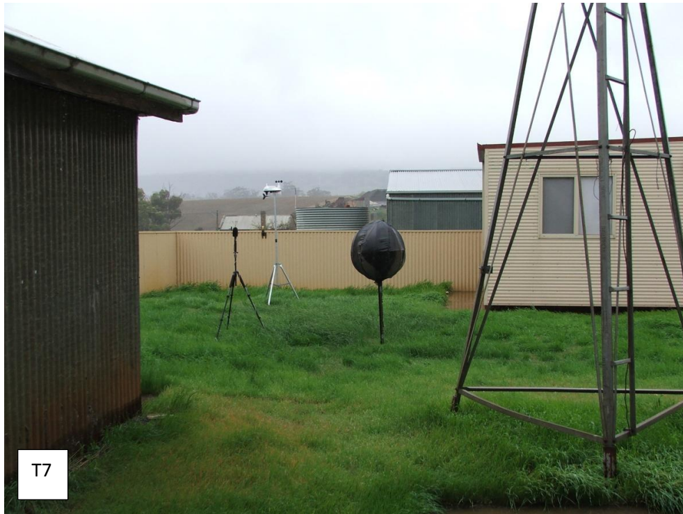
Figure T7: Township site - photo taken over corrugated iron fence looking East towards turbines (turbines not visible in low cloud). The distance between the ATCO hut and the garage is 9.4 m hence microphone is less than 5 m from any reflective surface – contrary to EPA guidelines.
